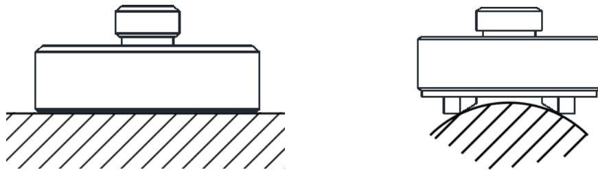
(a) Flat magnetic installation (b) Double-track (horseshoe-shaped) magnetic installation
